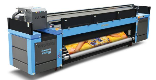
ColorJet **VULCAN** is a high speed 3.2 m roll-to-roll UV LED Inkjet printer. This back to back printing machine is used for printing banners, signage, billboards, terminal graphics, bus shelters, tradeshow graphics, window displays, backlit, wall graphics, building wraps, POP and POS graphics, etc. It is equipped with the capability to print 3-layer, 4-layer, and 5-layer printing. LED lamps and UV inks list this industrial UV printing machine.
